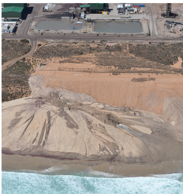
Collapse of the sea cliff below the Tormin processing plant on the West Coast of South Africa.
